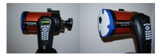
**Fig. 11** Experimental sensor setup consists of a Celestron® NexStar® 6SE 1.5 m focal length telescope with a mask to reduce the aperture to 5 cm, and an Orion® Starshoot<sup>™</sup> G3 mono-chrome camera.
