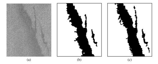
Fig. 4 Performance of the Markov random fields (MRF) algorithms using an image subset of 150 × 180 pixels: (a) subset of the original synthetic aperture radar (SAR) window of April 26, (b) result of a conventional MRF segmentation, and (c) result of the proposed new MRF scheme.
