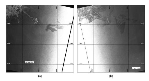
Fig. 2 Geo-referenced ASAR wide swath images of the Deepwater Horizon oil spill after projection onto an equidistant cylindrical projection: (a) April 26 and (b) May 2.
