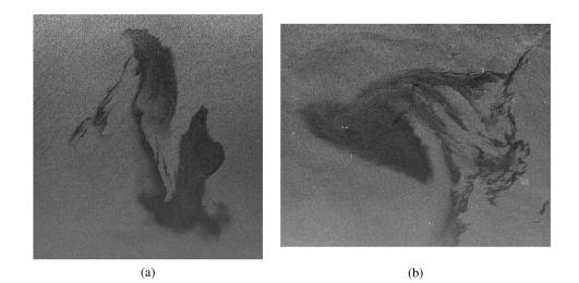
Fig. 3 Test images as subsets of the two ASAR raw images after correction of the slant range effect on the backscatter: (a) April 26 and (b) May 2.
