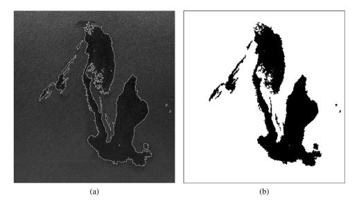
**Fig. 6** Segmentation results with the image of Fig. 2(a): (a) with the contour between the two regions of interest, oil spill and sea, overlapped to the original image and (b) binary detection with data of Fig. 2(a).
