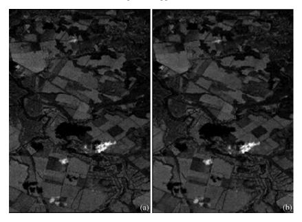
Fig. 8 Fragments of (a) original and (b) compressed image in 220'th sub-band.
