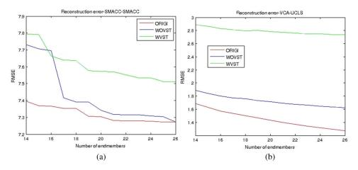
Fig. 13 RMSE versus (a) endmembers number for VCA and UCLS or (b) SMACC approaches for three considered sub-images, Original, WOVST, and VST lossy compressed.
