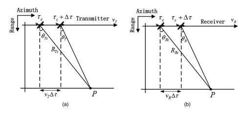
**Fig. 2** The flight geometry of transmitter and receiver. (a) The geometry of transmitter's track. (b) The geometry of receiver's track.
