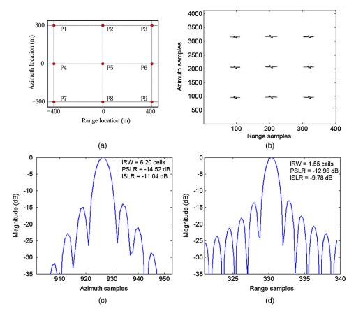
**Fig. 5** CSA imaging results based on the bistatic point target reference spectrum obtained by MLBF. (a) The locations of simulated targets. (b) The contours of final imaging result with 30 dB dynamic range. (c) The azimuth profile of the target P9. (d) The range profile of the target P9.
