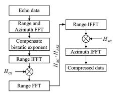
Fig. 3 Block diagram of chirp scaling algorithm (CSA) used in bistatic forward-looking SAR.
