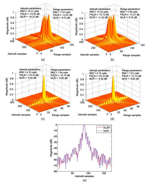
Fig. 4 Focusing results. (a) Processing result using Loffeld's bistatic formula (LBF).
