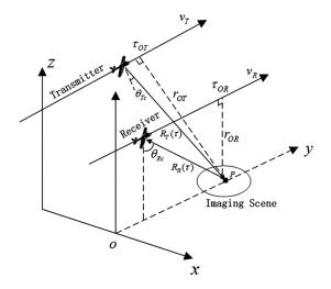
Fig. 1 The geometry of bistatic forward-looking synthetic aperture radar (SAR).
