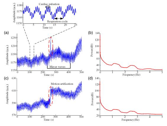
**Fig. 5** The raw optical signals of 760 and 850 nm recorded from one channel. (a) and (c) The optical signal of 760- and 850-nm wavelength, respectively. The signals were downsampled to 10 Hz. (b) and (d) The power spectra of optical signal of 760- and 850-nm wavelength, respectively.
