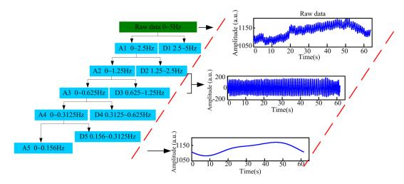
Fig. 6 The decomposition schematic diagram of a DSWT to the raw optical signals. The hemodynamic signal component localized in the approximation component of level 6 (0 to 0.156 Hz). The detail components of D2 and D3 are used for CTHR calculation.
