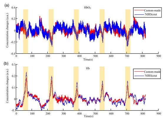
Fig. 4 Comparison of the time course of (a)  $HbO_2$  and (b) Hb acquired from NIRScout and a custommade device during Valsalva maneuver task.
