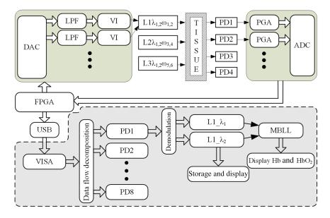
Fig. 2 The hardware and software architecture of the multichanneled fNIRS system. The hardware platform consists of a DAC and LED-driver module, a PGA and ADC module, and an FPGA controller and USB interface module. The function of the LabVIEW software system consists of USB data reading, data flow decomposition, signal demodulation, cerebral hemodynamic information calculated based on the MBLL, signal display, and storage.
