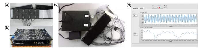
Fig. 3 The display of the multichanneled fNIRS system. (a) The wearable headset, (b) the disassembled prototype of the hardware motherboard, (c) the device appearance with the size of 125 mm  $\times$  110 mm  $\times$  50 mm, and (d) the software interface developed based on Labview.
