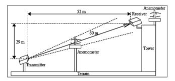
Fig. 1 Sketch of FSO link of the IAP Prague at Milesovka hill.
