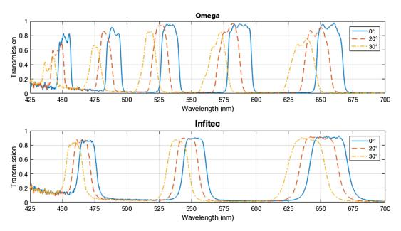
Fig. 6 Drift as a function of viewing angle measured on Omega filters and Infitec filters.
