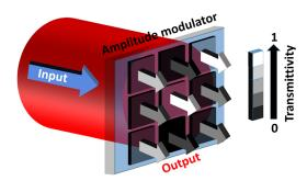
Fig. 4 Amplitude modulation of a light beam using a SLM with varying transmittivity across the beam cross-section.
