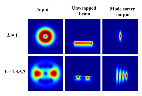
Fig. 35 The simulation results for various OAM mode inputs.
