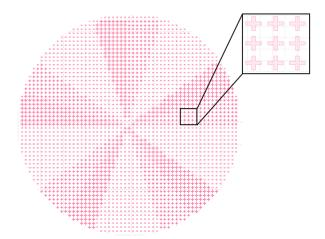
**Fig. 20** GDSII layout of an SPP for generation vortex beam ( $\ell = 5$ ) based on cylindrical-type meta-atom. The increase in the size of the cross gives a transmission phase of 0 to  $2\pi$ .
