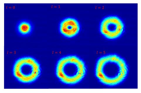
Fig. 18 Intensity profiles of zero-radial order OAM modes.
