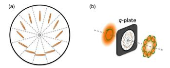
**Fig. 23** (a) Structure of the segmented q=1/2 plate, with indication of the LC director orientation. (b) Q-plate transforms right circularly polarized beam into left circularly polarized beam with an azimuthal phase  $\exp(i\phi)$  (reprinted from Ref. 124).
