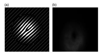
Fig. 27 Lee pattern and output for a  $400 \times 400$  pixel LG1 beam: (a) pattern generated using Lee holography and (b) experimental output of Lee holography.
