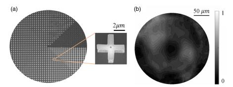
**Fig. 22** (a) SEM image of meta-SPP for I = +1 topological charge; the inset shows the single building block. (b) Vortex beam image captured on the  $64 \times 64$  pixel FPA detector (reprinted from Ref. 112).
