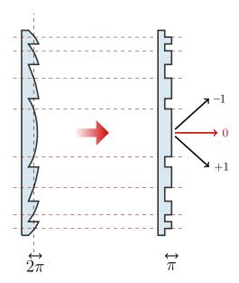
Fig. 8 Conversion from a Fresnel lens to a diffractive lens by quantizing the phase levels to binary levels (0 and  $\pi$ ).
