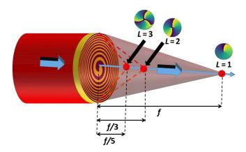
Fig. 12 Generation of spiral phases at different axial distances of a binary spiral Fresnel zone plate.
