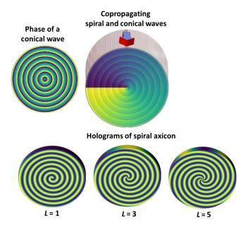
Fig. 16 Formation of spiral axicon hologram from interference between a spiral wave and a conical wave.
