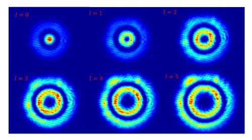
Fig. 19 Intensity profiles of first-radial order OAM modes.
