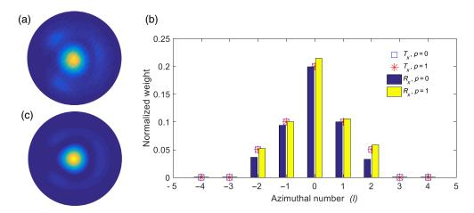
**Fig. 38** (a) Intensity structure of the generated composite beam consisting of 10 LG modes. (b) Weights of the generated (markers) and decomposition (bars) LG mode spectrum for radial orders p=0, 1 plotted as a function of different azimuthal mode indices l=-4 to +4. (c) Intensity structure simulated using the experimentally obtained modal weights.
