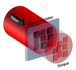
Fig. 3 Phase modulation of a light beam using an SLM with varying phase across the beam cross section.
