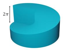
**Fig. 6** SPP for generation of LG beam with  $\ell = 1$ .
