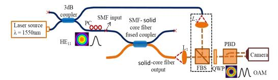
**Fig. 30** Experimental setup for characterizing the generated OAM beam: solid lines are propagation path of light through the fiber; dashed lines are that of light through free space. PC, polarization controller; L1 and L2, collimating lens; FBS, free space beam splitter; QWP, quarter waveplate; and PBD, polarization beam displacer.
