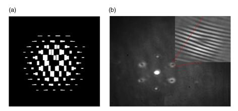
**Fig. 29** Experimental output of binary Fraunhofer holography: (a) pattern for LG1 beam and (b) interference of  $LG_{10}$  beam and a reference beam.
