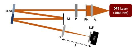
**Fig. 36** Experimental setup for implementing the optical correlation technique. DFB, distributed feedback laser;  $L_1$  (focal length = 10 cm) and  $L_2$  (focal length = 20 cm), convex lens; PH, pinhole; P, polarizer; SLM, spatial light modulator; M, mirror; LLF, laser line filter at 1064 nm; CCD, charge-coupled device camera.
