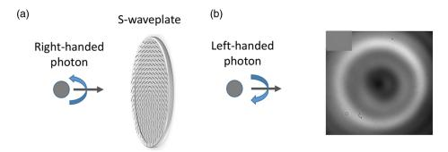
**Fig. 24** (a) Light with right circularly polarization and no OAM transmitted through the S-waveplate changes to left circularly polarized OAM beam. (b) Measured intensity profiles of left circularly polarized OAM beam (reprinted from Ref. 21 with the permission of AIP Publishing).
