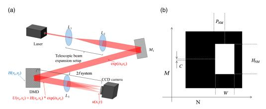
Fig. 28 Binary Fraunhofer holography method: (a) schematic representation of binary Fraunhofer holography method and (b) cell.
