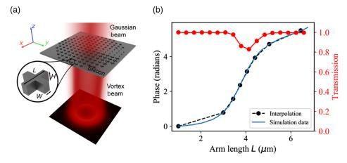
**Fig. 21** (a) Schematic representation of the vortex generator layout, silicon cross meta-atom in the inset. (b) Lookup table for IR cross resonators: the length L of the cross arm is varied from 1 to 6.5  $\mu$ m to achieve 0 to  $2\pi$  transmission for IR design (reprinted from Ref. 112).
