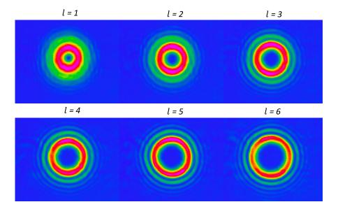
**Fig. 17** OAM modes of azimuthal order *l* from 1 to 6 generated using the sinusoidal gratings programmed in the SLM.
