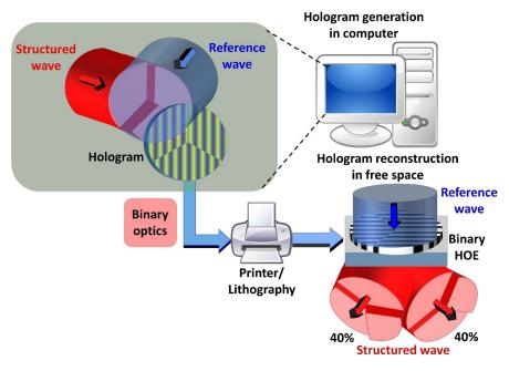
Fig. 10 Hologram recording within computer and reconstruction in free space.
