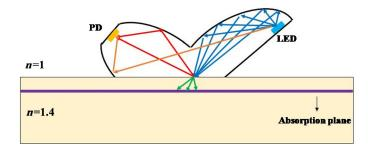
Fig. 7 A skin model without scattering effect is built to calculate the invalid light energy.
