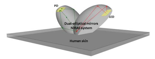
Fig. 5 Structure of a dual-elliptical mirrors NIRAS system.
