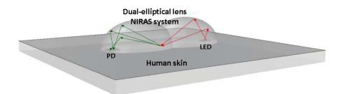
Fig. 2 Structure of the dual-elliptical lens NIRAS system. The dual-elliptical lens can help to focus the emitting light beam and collect backscattering light.
