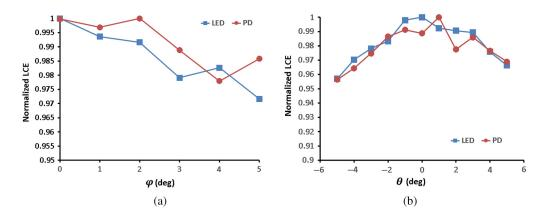
**Fig. 12** Rotating tolerance analysis of the LED and PD. The corresponding normalized LCE in the (a)  $\varphi$  direction and (b)  $\theta$  direction.
