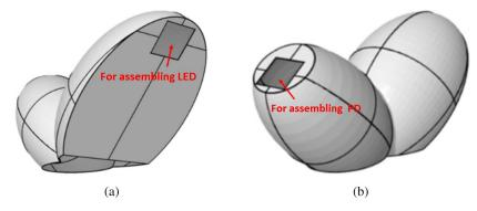
Fig. 10 Two square holes with 1-mm<sup>2</sup> area are designed for easily assembling LED and PD: (a) for assembling LED and (b) for assembling PD.
