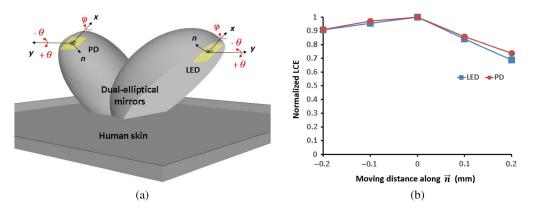
Fig. 11 Shifting tolerance analysis of the LED and PD: (a) coordinate axis setup of the dualelliptical mirrors NIRAS system and (b) comparison of the normalized LCE with the displacements of LED and PD.
