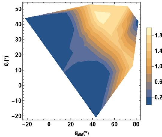
**Fig. 11** Results of fitting  $\text{BRDF}(\theta_{\text{BB}}, \theta_r) = f_{\text{surf}}(\theta_{\text{BB}}, \theta_r) + \rho_{\text{DDR}}(\theta_{\text{BB}}, \theta_r)/\pi$  (units of  $\text{Sr}^{-1}$ ) of Eq. (15) to the diffuse-sample data.
