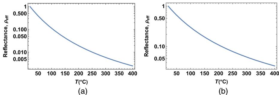
**Fig. 6** Constant band-integrated radiance,  $\rho_{\text{eff}} \int_{\Delta\lambda} L_{\text{BB}}(\lambda, T) d\lambda$ , makes solution of  $(\rho_{\text{eff}}, T)$  nonunique. (a) MWIR, 3.3 – 5.6  $\mu\text{m}$ ,  $L(\rho_{\text{eff}}, T) = 310 \mu\text{W cm}^{-2} \text{Sr}^{-1}$ . (b) LWIR, 5.6 to 12.5  $\mu\text{m}$ ,  $L(\rho_{\text{eff}}, T) = 5.3 \text{ mW cm}^{-2} \text{Sr}^{-1}$ .
