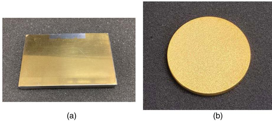
**Fig. 7** Reflectance samples used. (a) Polished Al, aka the “specular” sample, and (b) flamed-sprayed Al, aka the “diffuse” sample, both with Au deposited on them.
