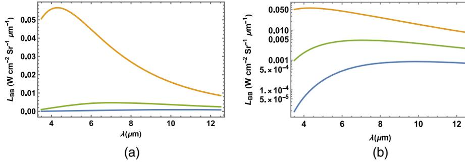
**Fig. 3** Planck's radiation law [Eq. (8)]. (a) Linear plot and (b) log-linear plot with  $T = 500^\circ\text{C}$ ,  $136^\circ\text{C}$ , and  $20.5^\circ\text{C}$  (top to bottom) and peak wavelengths at  $\lambda_{\text{peak}} = 4.3$ ,  $7.1$ , and  $9.9 \mu\text{m}$ , respectively.
