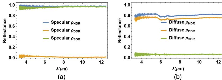
**Fig. 8** At  $40 \text{ deg} \leq \theta_r \leq 50 \text{ deg}$ , (a) for the polished sample,  $\rho_{\text{HDR}} = 0.98 \pm 0.004$ ,  $\rho_{\text{DDR}} = 0.024 \pm 0.008$ , and  $\rho_{\text{SDR}} = 0.95 \pm 0.01$ , across the 3.3- to 12.5- $\mu\text{m}$  band, and (b) for the flame-sprayed sample,  $\rho_{\text{HDR}} = 0.81 \pm 0.02$ ,  $\rho_{\text{DDR}} = 0.75 \pm 0.02$ , and  $\rho_{\text{SDR}} = 0.06 \pm 0.006$ , across this band.
