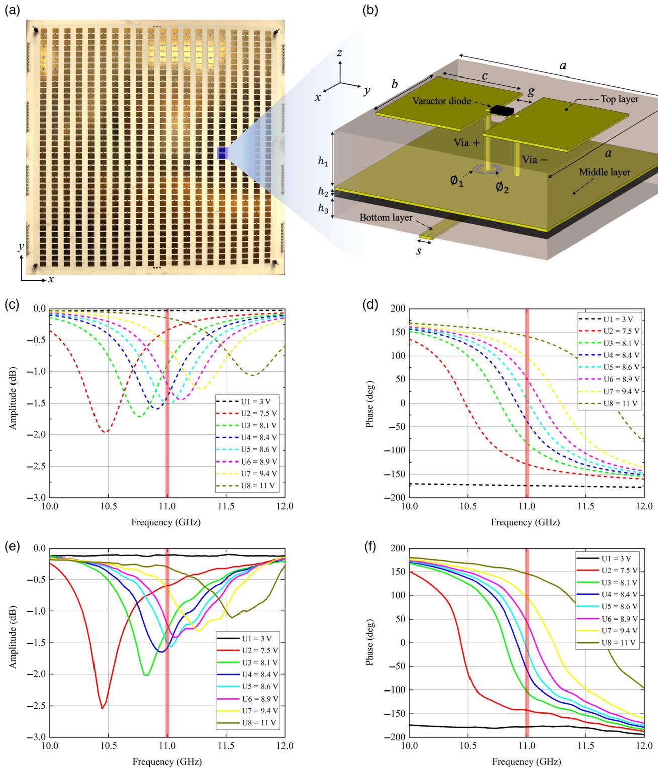
**Fig. 2** Metasurface design and reflection responses. (a) Photo of the fabricated space-time-coding digital metasurface. (b) Detailed geometrical parameters of the element structure. (c), (d) Simulated reflection amplitude and phase of the metasurface at different bias voltages, where the vertical orange line indicates the operating frequency at 11 GHz. (e), (f) Measured reflection amplitude and phase of the metasurface at different bias voltages.
