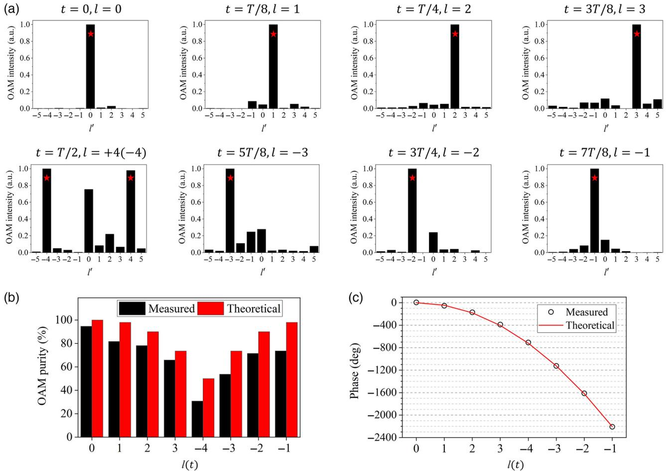
**Fig. 4** Spectrum analysis of time-varying OAM. (a) OAM intensity and phase spectrum of the measured time-varying OAM beams at different instants of time. (b) Measured and theoretical OAM mode purity for the dominant  $l(t)$ . (c) Comparison of measured and theoretical twisting phases for different time instants of dominant  $l(t)$ .
