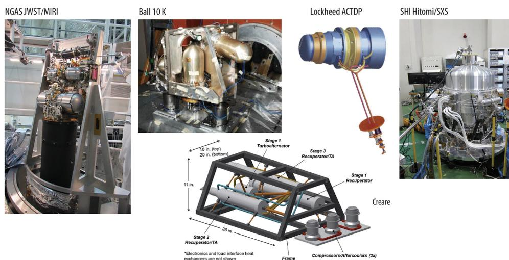
**Fig. 3** Five vendors have developed cryocoolers that have reached TRL 4+ and need only small improvements to meet the Origins's requirements.
