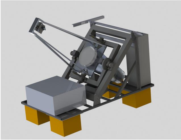
**Fig. 1** PICTURE C uses a 60 cm clear aperture, off-axis, Gregorian telescope in the Wallops ArcSecond Pointing (WASP) system. The clear aperture system allows PICTURE C to implement a high-performance vortex coronagraph while the use of the WASP system provides high pointing precision at low cost.
