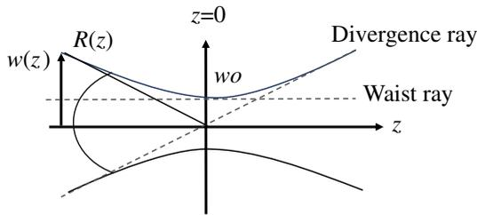
**Fig. 2** Gaussian beam  $1/e^2$  point curves shown near waist, with divergence and waist rays indicated.
