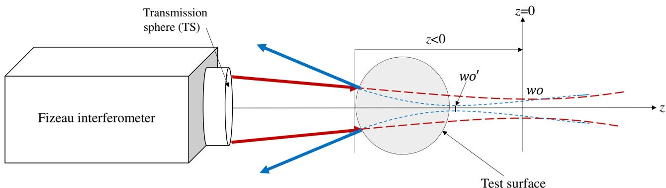
Fig. 6 The interferometer system being modeled, from TS to test ball back to TS.
