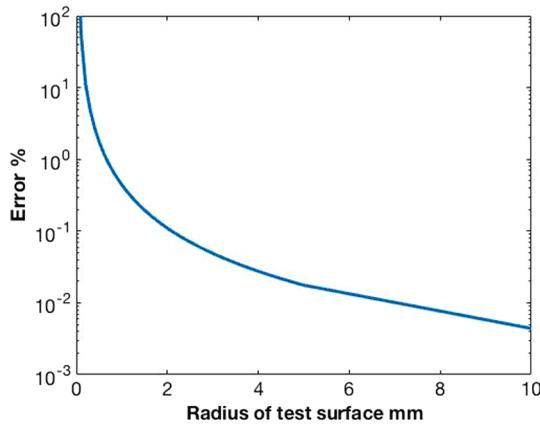
**Fig. 9** The percent error in logarithmic scale of the measured radius of curvature using the null to cat's eye test.
