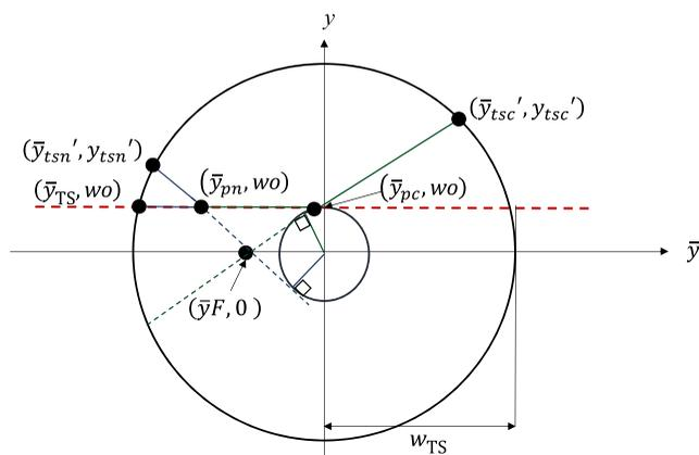
Fig. 7 The yybar diagram for both the null and cat's eye positions, from TS to test ball back to TS'.
