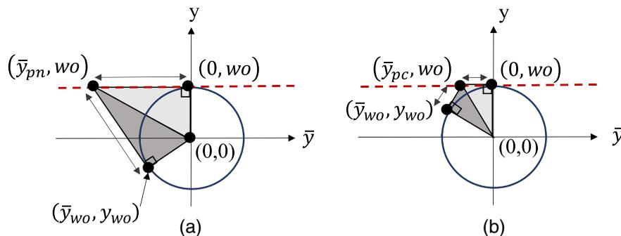
Fig. 8 Area is proportional to distance in a yybar diagram, so the triangles show the distance from the ball surface to the incident or reflected waist is identical for the (a) null or (b) cat's eye position; the reflected and incident waists are coincident.
