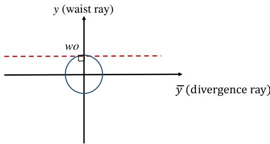
**Fig. 3** A yybar diagram, red dashed line, for the propagating beam in Fig. 2. Note that line is tangent to blue circle of radius  $w_0$ .
