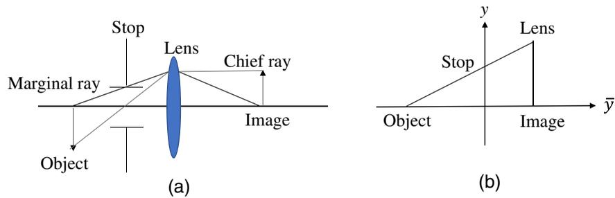
**Fig. 1** (a) Marginal and chief rays given a simple lens with the stop near the FFP. (b) The yybar diagram for the same lens system.
