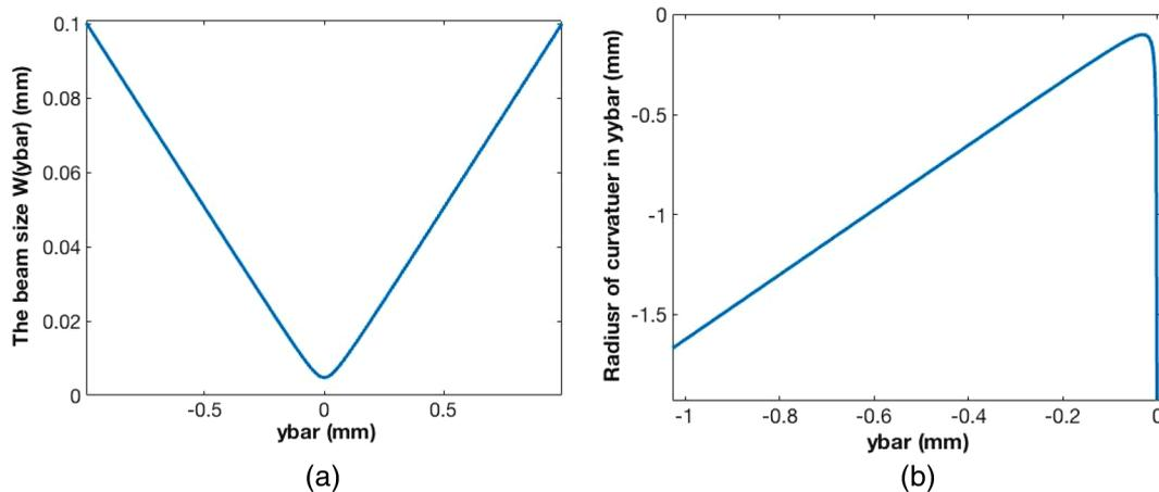
**Fig. 4** (a) The beam width,  $w(\bar{y})$ , through the waist and (b) radius of curvature,  $R(\bar{y})$ , up to the waist for the Gaussian beam in Fig. 3.
