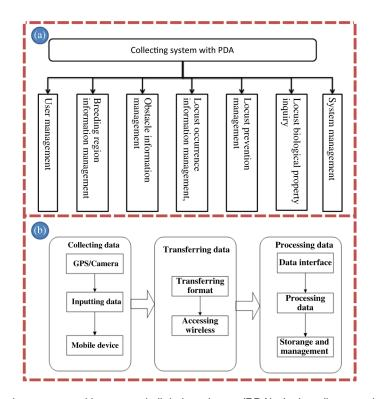
Fig. 4 Collecting system with personal digital assistant (PDA) design diagram. (a) Collecting system with PDA function diagram. (b) Working flowchart of collecting system with PDA.
