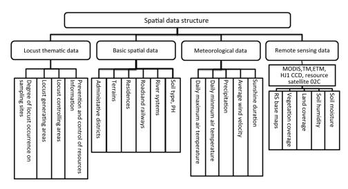
Fig. 3 Spatial database structure diagram.
