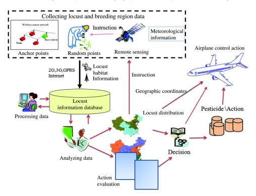
Fig. 1 Technical route of a monitoring and controlling system for locusts.
