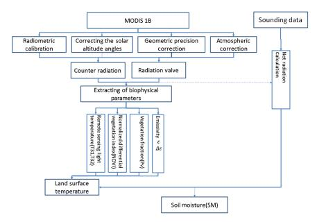
Fig. 8 Flowchart of MODIS 1B data processing.
