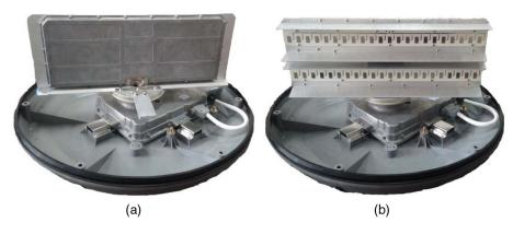
Fig. 8 The scanning radar system [(a) front side and (b) back side] utilized to collected scattering data.
