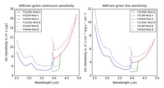
**Fig. 3** (a) Point-source continuum and (b) emission line sensitivities are shown for grisms with F322W2, F410M, and F444W filters for both modules A and B. Note that the narrower bandwidth of the F410 filters results in significantly better sensitivity than the wider F444W at common wavelengths.
