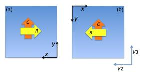
**Fig. 4** Grism dispersion orientations along detector axes (x,y) and the JWST observatory axes (V2,V3). The V3 position angle is defined to be 0 deg when V2 points east and V3 points north in the sky. The yellow and orange arrows point in the direction of increasing wavelength for R and C grisms in (a) module A and (b) module B, respectively. Each module has a  $2.'2 \times 2.'2$  imaging FOV.
