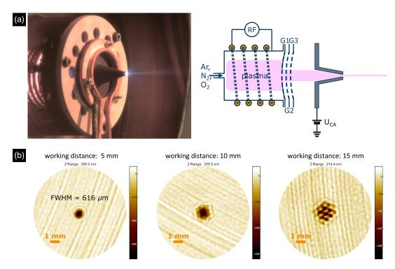
**Fig. 7** (a) Ion beam source with attached contraction aperture. The exit pupil diameter is 0.885 mm. (b) Interferometer images of footprint etchings in Al905 from a 1.5-keV nitrogen ion beam at different working distances.
