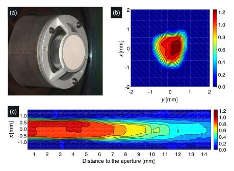
Fig. 6 (a) Ion beam source with attached pinhole aperture. The pinhole diameter is 0.8 mm. (b) Crosssectional Faraday probe measurement of an 1.5-keV oxygen ion beam at 0.5 mm distance to the aperture and corresponding (c) in-plane Faraday probe measurement.
