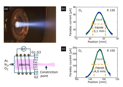
**Fig. 3** (a) TCP-type ion beam source with concave-shaped extraction grids (curvature radius R) resulting is a constriction of the ion beam. (b/c) Faraday probe measurements of 1.5-keV oxygen ion beams at the working distance for grid curvature radius (b) R = 150 mm and (c) R = 100 mm.
