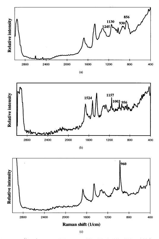
Fig. 30 FT Raman spectra of human brain tumors at 1064 nm excitation (200 to 300 mW, 1000 to 3000 scans): (a) glioma grade III, (b) acoustic neurinoma, and (c) central neurocytoma. (Modified from Ref. 69.)
