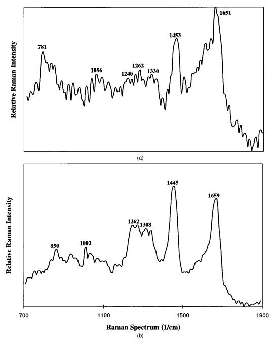
Fig. 35 FT Raman spectra of human ovarian tissue at 1064 nm excitation (1 W, 800 scans): (a) malignant ovarian tissue and (b) normal ovarian tissue. (Modified from Ref. 8.)
