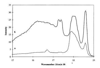
**Fig. 38** Raman and luminescence spectra at 488 nm excitation of (a) core in a 200  $\mu$ m core optical fiber from Diaguide and (b) cladding and buffer of the same optical fiber. (Modified from Ref. 76.)
