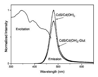
Fig. 1 Excitation and emission spectra for  $CdS/Cd(OH)_2$  QDs and functionalized  $CdS/Cd(OH)_2$ -glutaraldehyde QDs.
