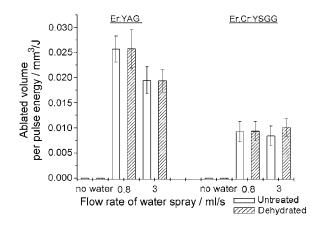
**Fig. 3** Ablated volume in dental enamel as a function of pulse energy (ablation efficiency), plotted against the flow rate of the externally supplied water spray.
