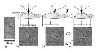
**Fig. 2** Directional control of a rigid fine rod. The scale bar is 20  $\mu$ m for the pictures. (a) The target fiber on the glass plate. The fiber is less than 1  $\mu$ m thick, and is observed as a dark line. (b) The fiber is trapped along the focused laser. The fiber is vertical with respect to the observation field. (c) The tilted fiber along the laser axis. (d) The tilted fiber,  $\Delta \varphi = 90$  deg, with respect to (c).
