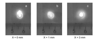
**Fig. 7** Diameter and distribution of plasma emission in the plasmamaterial interaction zone depending on the distance x of the nozzle to the quartz plate surface for (a) x=0 mm, (b) x=1 mm, and (c) x=3 mm.
