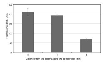
**Fig. 8** Intensity of the plasma emission on the distance of the nozzle to the guartz plate surface.
