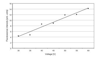
Fig. 3 Influence of the applied voltage on the plasma intensity in the plasma stream.
