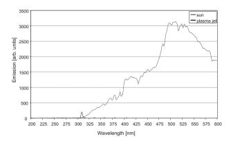
Fig. 11 Spectral intensity of the sun compared to the spectral distribution of the plasma jet.
