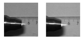
Fig. 4 Influence of the applied gas pressure on the length of the plasma stream.
