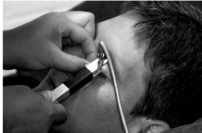
Fig. 2 The wand device being used to measure eyelid spectral transmittance. The LED is positioned under the eyelid and the detector above the eyelid.
