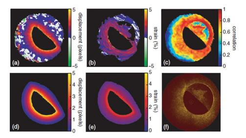
**Fig. 5** (a) Displacement and (b) strain fields resulting from the ALE algorithm, and the value of (c) the correlation coefficient. The data in (a) and (b) may be compared to the simulated data (d) and (e) used for input. (f) The OCT image used for the simulation (Ref. 75). Reproduced with permission from IOP.
