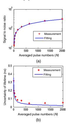
**Fig. 3** Signal-to-noise characterization of system performed on fluorescein decays with different number of averaged pulses (N=5, 10, 20, 40, 80, 160, 320, 640, 1280, and 2000). (a) SNR increased following a linearly proportional to  $\sqrt{N}$  as predicted by the Poisson distribution as the fitting curve shows. (b) Standard deviation (uncertainty) of lifetime decreased with the increase of averaged pulse numbers, which is inversely proportional to  $\sqrt{N}$ .
