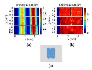
**Fig. 4** Effects of the scanning steps on the spatial resolution (image quality). The intensity (a) and lifetime (b) images of fluorescence phantom #1 at 515 nm are measured at three different scanning steps (top to bottom: 0.1, 0.2, and 0.3 mm). (c) A schematic view of phantom #1. A pair of capillary tubes filled with fluorescein dyes embedded into the phantom matrix in parallel. The distance between two capillary tubes is 1 mm.
