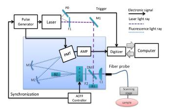
**Fig. 1** A schematic view of the acousto-optic tunable filter (AOTF)-based hyperspectral fluorescence lifetime imaging (FLIM) instrument. M1: flat mirror; M2, M3: concave mirrors; DM: dichroic mirror; C1: plano-concave lens; F1: neutral density filter; F2: long-pass filter; B1, B2: beam stops; PD: photodiode; AOTF: acousto-optic tunable filter; MCP-PMT: multichannel plate photomultiplier tube; AMP: preamplifier.
