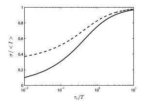
**Fig. 7** Theoretical speckle contrast as a function of the ratio of the speckle correlation time to exposure time, for a completely dynamic medium (solid line) and a medium with a fraction of stationary scatterers (broken line) (schematic only).
