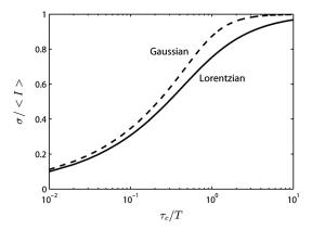
**Fig. 6** Theoretical relationship between speckle contrast and the ratio of the speckle correlation time to exposure time, assuming a Lorentzian and a Gaussian velocity distribution, respectively. (Note that  $\beta$  has been set to 1 and the two curves have been normalized so that they can be compared.)
