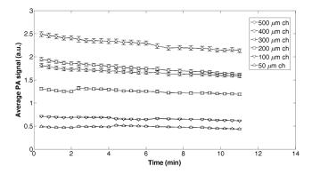
Fig. 6 PA average signal acquired with P1 loaded with ICG solution 1 mM, irradiated for 11 min; each curve is relative to a channel (ch).
