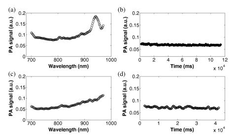
Fig. 3 Absorption spectrum and photoacoustic (PA) signal during time of [(a) and (b)] P2 and [(c) and (d)] P1 filled by water.
