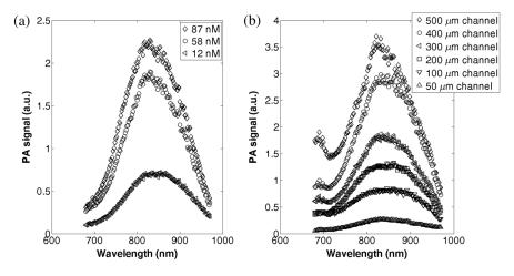
**Fig. 8** (a) Absorption spectrum of PEG-GNRs at three different dilutions (87, 58, and 12 nM) in P2 and (b) PEG-GNRs 87 nM in P1; each curve is relative to a channel.
