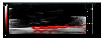
Fig. 4 PA images of P1 loaded with indocyanine green (ICG) solution 1 mM. B-mode image (gray levels) and PA signal (red) are superimposed.
