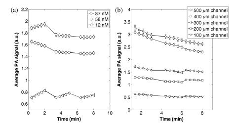
**Fig. 10** PA average signal of PEG-GNRs, acquired during 8 min, loaded (a) in P2 (87 nM rhombus, 58 nM circles, 12 nM triangles) and (b) in P1 (500  $\mu$ m channel rhombus, 400  $\mu$ m channel circles, 300  $\mu$ m channel left-pointing triangles, 200  $\mu$ m channel squares, 100  $\mu$ m channel upward-pointing triangles), loaded with PEG-GNRs, irradiated for 8 min.
