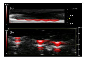
**Fig. 7** (a) PA images of P1 loaded with PEG-GNRs 87 nM and (b) P2 loaded with PEG-GNRs at three different dilutions: 87, 58, and 12 nM. B-mode image (gray levels) and PA signal (red) are superimposed.
