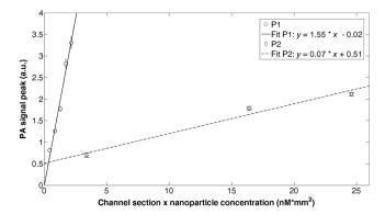
**Fig. 9** Peak signal versus nanoparticle concentration multiplied by the channel section for P1 loaded with PEG-GNRs 87 nM (circles and continuous line) and for P2 loaded with PEG-GNRs at three different dilutions (87, 58, and 12 nM) (rhombus and dotted line).
