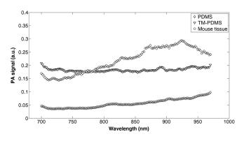
**Fig. 12** Absorption spectrum of PDMS (rhombus), TM-PDMS (downpointing triangles), and mouse tissue (region of mouse spleen at 2 mm of depth under the skin) (circles).
