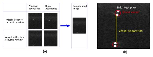
**Fig. 7** (a) Four PA frames show four different vessel boundaries, representing two blood vessels. These four frames were compounded in a single image. (b) The brightest pixel at each boundary in the compounded image was used to compute vessel separation.
