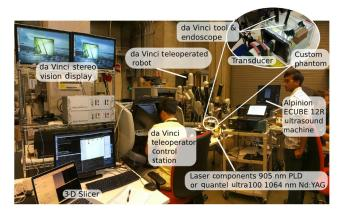
**Fig. 3** Physical setup when interfacing our PA imaging system with the da Vinci Surgical System. The inset image shows the custom-built phantom. The US transducer was oriented orthogonal to the vessels for this experiment.
