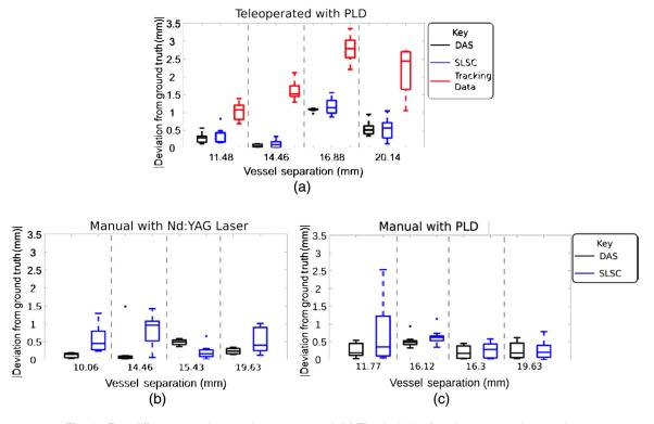
**Fig. 10** Four different vessel separations were tested. (a) The deviation from known vessel separations was measured using tracking data from the da Vinci and PA images acquired with the PLD. Similar results were obtained when manually sweeping an optical fiber coupled to the (b) Nd:YAG laser and (c) PLD.
