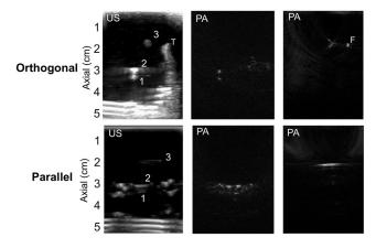
**Fig. 12** Sample US and PA images demonstrating vessels 1 to 3 in orthogonal and parallel orientations. The tissue thickness for these US and PA images is 1.5 mm. All PA images were acquired with  $\sim$ 1.58-mJ energy at the tip of the fiber (T = tissue and F = signal from fiber).
