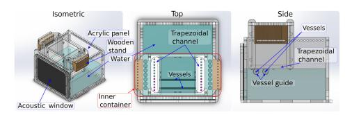
**Fig. 4** Overview of the phantom design, which consisted of acrylic panels, a rubber acoustic window for US signal reception, and plastic guides to control the vessel separation distances. The two black lines inside the phantom (top view) show a sample arrangement of parallel blood vessels. The phantom was filled with water for PA imaging. The US probe (not shown) was oriented orthogonal to the vessels for this experiment.
