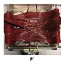
**Fig. 5** (a) Experimental setup to image a rigid 3-D printed vascular network combined with the flexible vessel from the previous set of experiments. (b) Experimental setup with tissue added to the vascular network phantom. The US probe was oriented both orthogonal (not shown) and parallel to the vessel axes for these experiments.
