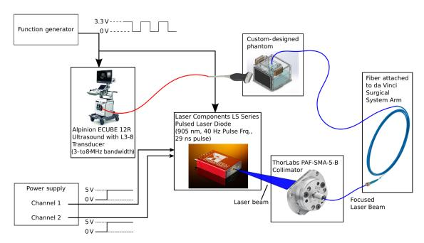
**Fig. 1** This configuration of our PA imaging system uses the PLD. The optical fiber was both handheld for manual operation and teleoperated when attached to one of the da Vinci surgical tools. A similar setup replaced the PLD with an Nd:YAG laser or Phocus Mobile laser.
