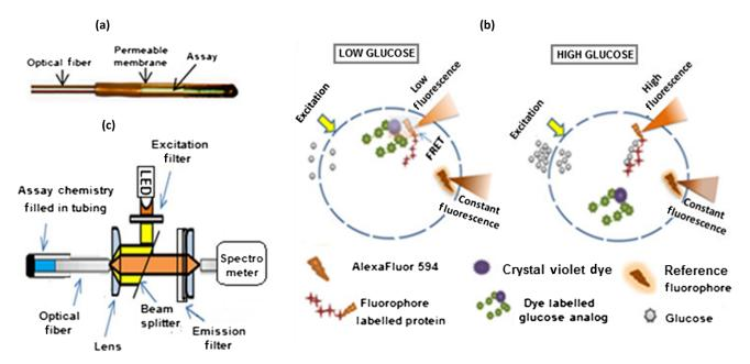
**Fig. 3** (a) Real glucose sensor. (b) Illustration of the assay chemistry and FRET sensing principle resulting in low and high intensity. (c) Optical setup for sensor characterization.
