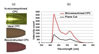
**Fig. 4** (a) From top to bottom: fs-laser micromachined CPC, ideal CPC, and reconstructed CPC shape in Zemax. (b) Average fluorescence spectra from plane-cut and micromachined CPC tips, each averaged over three measurements.
