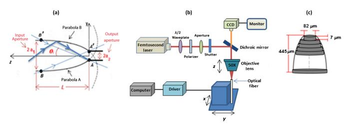
Fig. 2 (a) Geometry of a CPC. (b) is laser setup with stages to micromachine the fiber tip. (c) Illustration of carving process.
