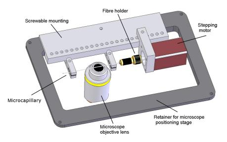
**Fig. 1** Device for rotation of 3-D samples (within microcapillaries) applicable to the x, y-stage of an inverted microscope (reproduced from Ref. 9 with modifications).
