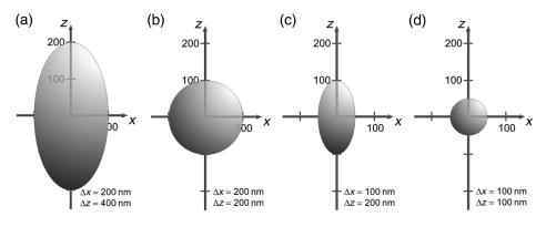
Fig. 6 (a) PSFs for conventional fluorescence microscopy, (b) axial tomography, (c) SIM, and (d) SIM in combination with axial tomography.
