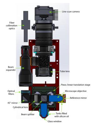
Fig. 2 Construction plan of the LC-OCT imaging head.
