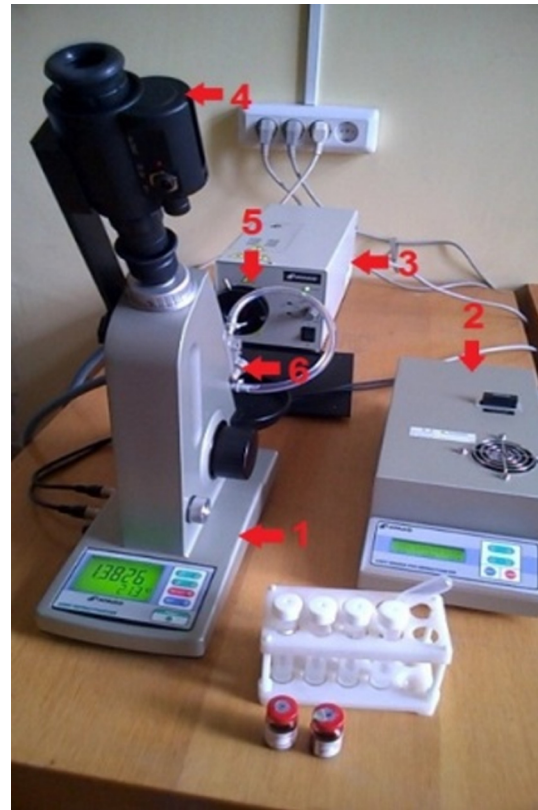
Fig. 1 General view of the multiwavelength Abbe refractometer (Atago, Japan): 1, refractometer; 2, power supply; 3, light source; 4, the eyepiece imager for measurements in the NIR region; 5, interference filter; and 6, sample.
