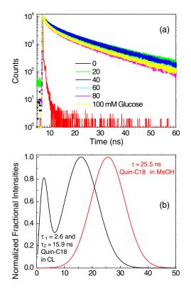
**Fig. 11** (a) Effect of glucose on the time-dependent decays of Quin-C18 in Comfilcon A lens. (b) Lifetime distribution of Quin-C18 in methanol and Quin-C18-labeled Comfilcon A lens.
