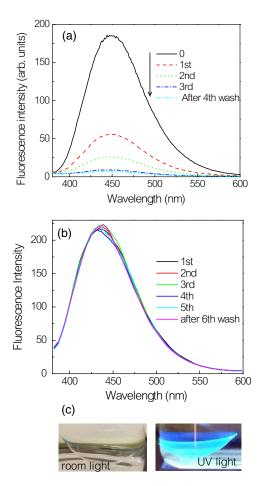
**Fig. 9** Emission spectra of (a) Quin and (b) Quin-C18 in a Comfilcon A contact lens with repeated washings. (c) Photograph of Quin-C18-doped Comfilcon A contact lens taken without an emission filter.
