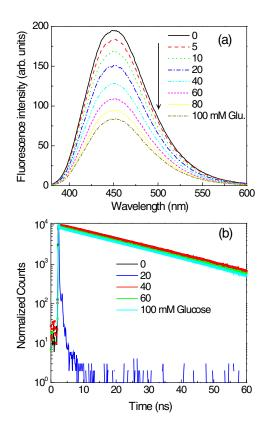
Fig. 8 Effect of glucose (a) on emission and (b) on emission intensity decays of Quin in pH 7.2 phosphate buffer.
