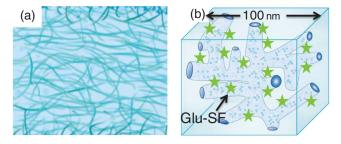
**Fig. 2** (a) Schematic cross section of HG contact lens showing the homogeneous interior structure. (b) Schematic of a small region of a SiHG showing the hydrophylic and hydrophobic IPNs. The dimension is an approximation.
