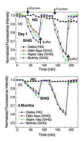
**Fig. 12** (a) Response of Quin-C18 to glucose or fructose within different SiHGs and in a HG in pH 7.2 phosphate buffer. Incrementing glucose concentrations (from 0 to 100 with 20 mM interval) and 0, 1, 2, 4, 7, and 10 mM of fructose were used before purging the lenses with final buffer. Bioaffinity, Aspire 1day, and OptixAqua are SiGHs and Dailies is a HG contact lens. (b) Similar response to the glucose or fructose from Quin-C18-doped lenses stored in water for 3 months.
