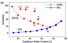
**Fig. 3** (a) Typical monomer used in a silicone HG contact lens. (b) Water content and Dk values of HG and SiHG lenses. LA, Lotrafilcon A; LB, Lotrafilcon B; G, Galyfilcon A; C, Comfilcon A; S, Stenfilcon A; and N, Nelficon A. Comfilcon A is a third-generation SiHG with improved Dk and high water content.
