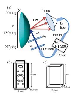
**Fig. 5** (a) Optical configuration for measuring fluorescence from surfaces of contact lens. BE, beam expander; VA variable aperture; and LD, laser diode. (b) Device to hold contact lens. (c) A  $2.5 \times 0.8$ -cm cuvette.
