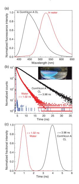
Fig. 6 (a) Emission spectra and (b) intensity decays of Prodan in a Comfilcon A contact lens or in water. Inset in (b) shows the labeled lens in a scintillation vial on a UV handlamp. (c) Lifetime distribution analysis of Prodan in water and Prodan-labeled Comfilcon A lens.
