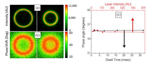
Fig. 7 (a) Effect of dwell time on accumulated intensity and phase angle, (b) effect of incident intensity on phase angle, and (c) summary plot for range of dwell time and laser intensity.
