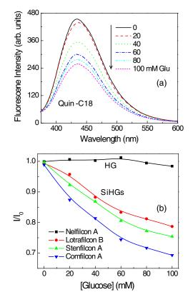
Fig. 10 (a) Glucose-dependent emission spectra of Quin-C18 within a Comfilcon A (Biofinity) SiHG lens. (b) Normalized emission intensities of Quin-C18 within a Nelfilcon A (HG) lens and that in three SiHG lenses: Comfilcon A (Biofinity), Stenfilcon A (Aspire 1day), and Lotrafilcon B (Optix Aqua) lenses.
