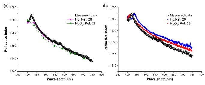
Fig. 4 The measured continuous CRID of hemoglobin solution, compared with (a) Ref. 27 and (b) Ref. 28.
