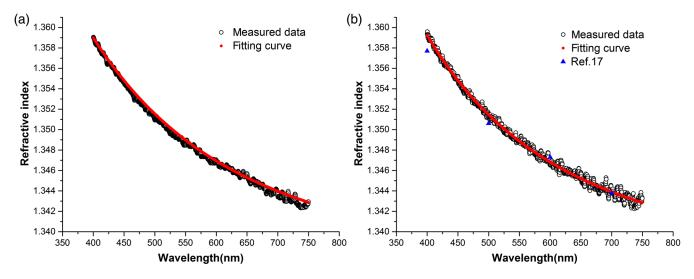
Fig. 2 The measured continuous CRIDs and fitting curves of (a) blood serum and (b) blood plasma.
