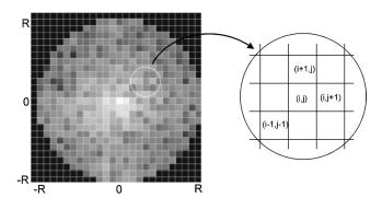
**Fig. 3** Matrix of the first-order Fourier spectrum selected from the Fourier-transformed interferogram. Right: the method of accessing the matrix elements by use of i and j indices for calculation of the second momentum of the first Fourier spectrum.
