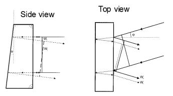
**Fig. 2** Side and top views of the wavefronts on the wedge.  $W_r$  represents the wavefront reflected from the first surface of the wedge, and  $W_i$  is the wavefront incident and reflected from the rear surface of the wedge.
