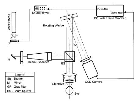
Fig. 1 The schematic setup of the lateral shearing interferometer.
