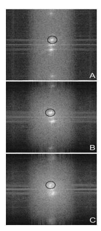
**Fig. 6** The Fourier spectra of the selections presented in Figures 5(a) through 5(c). The dark rings surrounding the first-order Fourier spectrum are selected for the second momentum calculation. The HIP is in the middle of the ring on each image.
