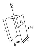
**Fig. 2** Direction of the eigenvectors of the moment of inertia of a hexahedron. The structure is assumed to be solid with a constant density function. a,b,c: the three sides,  $V_1$ ,  $V_2$ ,  $V_3$ : the main axes of inertia.
