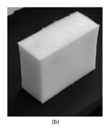
**Fig. 2** (a) The clear aqueous PVA solution in the Perspex mold carries the dyed, rigid PVA gel spheres suspended with nylon thread. The solution is allowed to stand at room temperature for a few hours to allow bubbles to rise to the surface, before it undergoes freezing and thawing cycles. (b) The resulting PVA gel breast phantom after submitting the solution to four freezing-thawing cycles.
