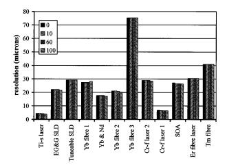
**Fig. 9** Change in resolution achievable in skin, without interaction with tissue (0), after returning from  $10-\mu$ m depth (10),  $60-\mu$ m depth (60), and  $100-\mu$ m depth (100).
