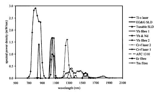
Fig. 4 Spectral intensity profiles of sources considered.
