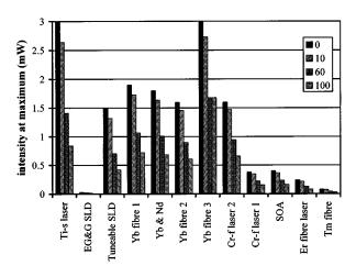
**Fig. 12** Change in intensity of source light in gallbladder, without interaction with tissue (0), after returning from  $10-\mu m$  depth (10),  $60-\mu m$  depth (60), and  $100-\mu m$  depth (100).
