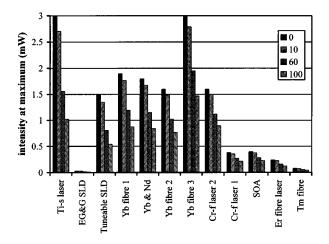
**Fig. 10** Change in intensity of source light in liver, without interaction with tissue (0), after returning from  $10-\mu$ m depth (10),  $60-\mu$ m depth (60), and  $100-\mu$ m depth (100).
