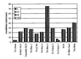
**Fig. 13** Change in resolution achievable in gallbladder, without interaction with tissue (0), after returning from  $10-\mu$ m depth (10),  $60-\mu$ m depth (60), and  $100-\mu$ m depth (100).
