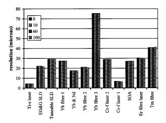
**Fig. 11** Change in resolution achievable in liver, without interaction with tissue (0), after returning from 10- $\mu$ m depth (10), 60- $\mu$ m depth (60), and 100- $\mu$ m depth (100).
