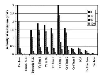
**Fig. 8** Change in intensity of source light in skin, without interaction with tissue (0), after returning from 10- $\mu$ m depth (10), 60- $\mu$ m depth (60), and 100- $\mu$ m depth (100).
