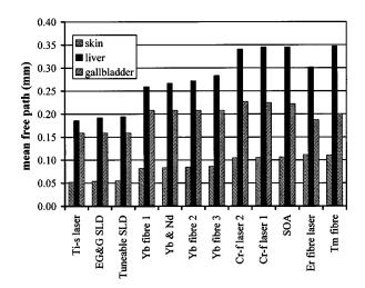
**Fig. 7** Mean-free paths in skin, liver, and gallbladder at the wavelengths of the maxima of the light sources. Ti-s, titanium:sapphire laser; SLD, superluminescent diode; Yb, fiber, superfluorescent ytterbium fiber; Yb and Nd, superfluorescent combination of Yb-doped and neodymium-doped fibers; Cr-f, chromium:forsterite laser; SOA, semiconductor optical amplifier; Tm fiber, superfluorescent thulium fiber.
