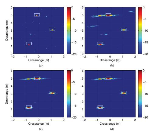
**Fig. 6** Scene images formed by different imaging approaches: (a) CS image formed by method in Ref. 10; (b) DS image formed by method in Ref. 12; (c) DS image formed by the proposed approach with wavelet dictionary; (d) DS image formed by the proposed approach with Gabor dictionary. All antenna locations are used and the frequency bins are just 20% of the total transmitted frequency. The signal is corrupted by the noise with SNR = 10 dB.
