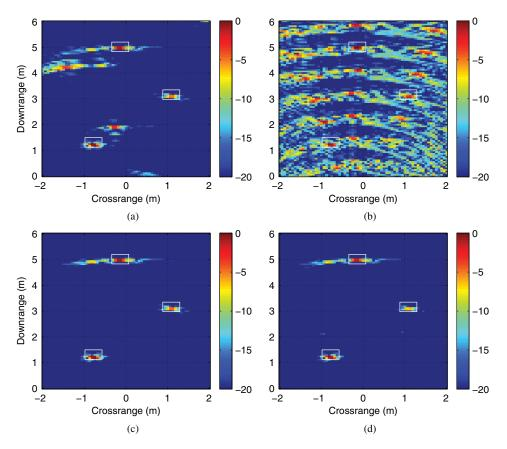
**Fig. 3** Scene images formed by different settings: (a) DS using 12% full data volume; (b) DS using 1% full data volume; (c) proposed approach using 12% full data volume. The signal is corrupted by the noise with SNR = 20 dB.
