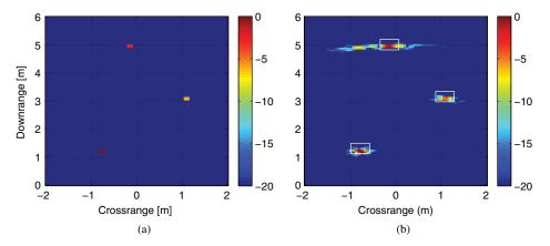
Fig. 2 The behind-the-wall scene space: (a) ground-truth image; (b) DS image formed using full volume of data samples.
