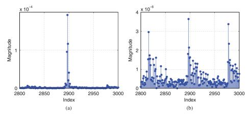
Fig. 10 Reconstructed signal coefficients **s** for the dihedral scene: (a) using the Gabor signal representation; (b) without using the Gabor signal representation.
