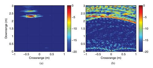
Fig. 8 Images formed by different settings: (a) conventional DS using full data volume; (b) conventional DS using 0.9% full data volume.
