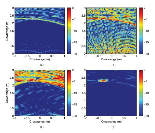
**Fig. 9** Images reconstructed by different imaging methods: (a) CS image by imaging method in Ref. 10; (b) DS image by imaging method in Ref. 12; (c) DS image by proposed approach without Gabor dictionary; (d) DS image by proposed approach with Gabor dictionary. The measurements constitute 0.9% of full data volume.
