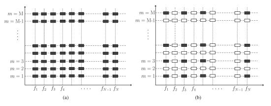
Fig. 1 Data acquisition for TWRI: (a) conventional radar imaging scheme; (b) TWRI based on CS. The vertical axis represents the antenna location, and the horizontal axis represents the transmitted frequency. The filled rectangles represent the acquired data samples.
