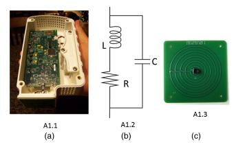
**Fig. 17** (a) Electronics, (b) coil, and (c) enclosure for the single-coil MIT imaging "scanner"; also, an equivalent circuit (b) representation for the coil sensor is shown.
