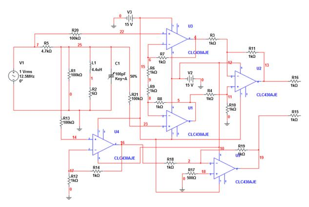
Fig. 18 Analog portion of circuit associated with coil (L1 in schematic); C1 is a tunable varactor, while R2 is the loss in L1—the quantity to be measured; outputs from R15 to R16 are used to drive the Analog Devices AD8302 phase-gain detector. Lower voltage OP amps were used in the actual instrument.
