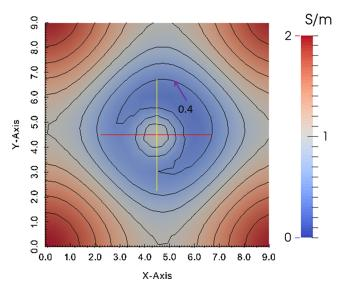
Fig. 4 Prescribed conductivity distribution used to create 61 virtual coil loss measurements using 4 cm diameter, 5-loop coil identical with that used in the study, over a 2-cm thick slab. Coil positions for sampling are noted in the text. Contours are shown at intervals of 0.2 S/m, with the contour at 0.4 given as reference.
