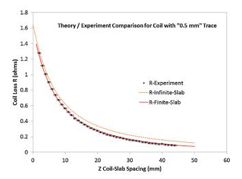
**Fig. 3** Comparing a theoretical prediction from Eq. (1) with measurement on coil with 0.5 mm trace. No data fitting or scaling is used here; rather, the comparison is "head-to-head." Also included is the infinite slab result [derivation not included, but similar to Eq. (1)].
