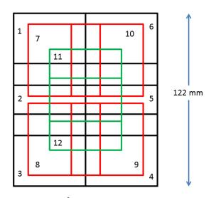
Fig. 7  $102 \times 122$  mm<sup>2</sup> template used for guiding placement of the MIT single coil—the PCB supporting the coil has square dimensions that allow it to just fit within any one of the squares.
