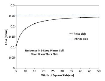
**Fig. 6** Impedance change in 5-loop coil (5 cm diameter) when positioned 1.0 mm above a 12-cm thick square slab of variable side dimension. The results are compared with the infinite slab value computed from an analytical formula. The finite element mesh used for computing impedance change from Eq. (1) has resolution of about 0.5 cm for slabs up to 30 cm along a side, thereafter 1.0 cm. Frequency is set at 12.5 MHz.
