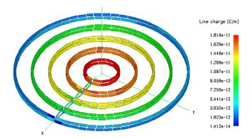
**Fig. 1** Geometry of two-layer, multiloop coil used for MIT imaging; loop radii—4, 8, 12, 16, and 20 mm; segment charges are shown for case with 1 V excitation at 12.5 MHz; 84 pF of capacitance and 20 k $\Omega$  of resistance were placed in parallel with the coil to resonate at 12.26 MHz; segment diameters were set at 0.6 mm to give a perimeter equivalent to that of a 1 mm, 2 oz. Cu PCB trace.
