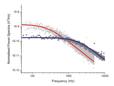
Fig. 13. The power spectrum of a trapped 100 nm gold (blue) and 100 nm polysterene (red) sphere can be fitted wit a Lorentzian curve. The curve fit provides the roll off frequency  $f_0$  for each particle in at a given power in a specific optical trap. The roll off frequency determines the trap stiffness  $\kappa$ .
