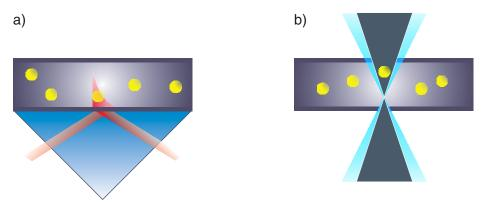
Fig. 6. a) Combining single-beam tweezers and evanescent fields lead to further insight in the interplay of scattering and gradient force components for metal nanoparticles [66]. b) A vortex trap is an alternative trapping geometry to single-beam tweezers [65]. The metal nanoparticle is confined in the dark vortex core of a Laguerre-Gaussian beam, avoiding the high intensity region of the laser.
