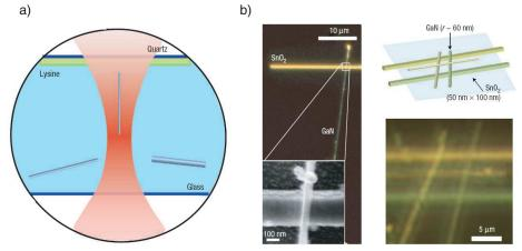
Fig. 3. a) The nanowires sink to the bottom of the sample chamber where they are picked up with optical tweezers, here pictured from the side. b) GaN nanowires and SnO2 nanoribbons optically laser-fused after they were manipulated in the correct place with optical tweezers. Pauzauski *et al.* imaged the nanowire structures with darkfield microscopy (see Sec. 4.4). Adapted from [48] and reprinted by permission from Macmillan Publishers Ltd: Nature Materials, copyright (2006).
