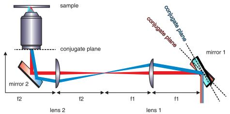
Fig. 9. Setting up the beam steering mirror nirror 1 at the conjugate plane of the back aperture of the trapping objective assures that the beam can be manipulated without walking of the back aperture of the objective. This allows moving the trapping position of the beam in the sample plane. At the same time the trapping laser always slightly overfills the back aperture of the microscope objective ensuring maximal axial as well as lateral trapping strength.
