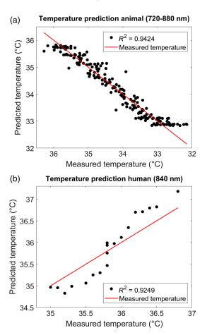
**Fig. 6** Temperature prediction. Predicted (brain) versus measured (rectal) temperature based on cross-validated PLSR. Plots exemplarily illustrate (a) the animal dataset (PIGLET02) during the cooling phase (wavelength interval 720 to 880 nm with three PCs) and (b) the human dataset (BABY01) during the rewarming phase (wavelength 840 nm with three PCs). See Table 4 for statistics.
