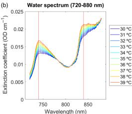
**Fig. 1** Temperature dependence of water spectrum. Extinction coefficient of pure water spectra ( $H_2O$ ) simulated as a function of temperature (range 30°C to 40°C) over NIR: (a) 600 to 980 nm and (b) 720–880 nm.<sup>7,8</sup> Pronounced water absorption peaks appear in the NIR around 740, 840, and 970 nm (marked by red vertical lines). Units are given in temperature (°C) with increasing extinction indicating increasing temperature (color coded from blue to red).
