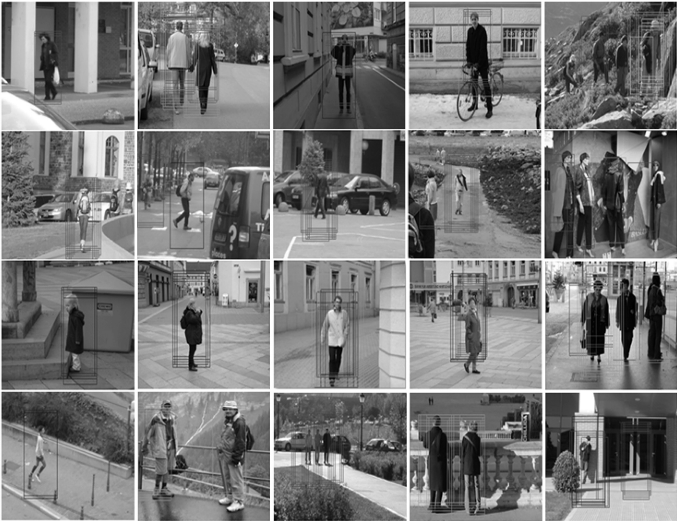
Fig. 6 Sample human detection results using INRIA images with the proposed method. The final column shows some false and misidentified results. Red box represents detected results from one-level wavelet-transformed image, blue box represents detected results from downsampling by a ratio of 0.8, green box represents detected results from downsampling by a ratio of 0.6, and yellow box represents detected results from upsampling by a ratio of 1.2.
