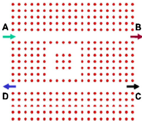
Fig. 4 Schematic structure of square shape photonic crystal ring resonator (PCRR) based ADF.
