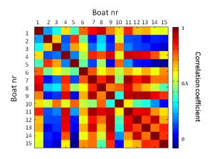
Fig. 15 The correlation matrix between boat profiles with no detector noise. The separation capability between the larger boat (no. 1 to 5) is better than for the smaller boats (especially boats 10 to 15). The value of the correlation coefficient is color coded as shown by the color bar (0 to 1).
