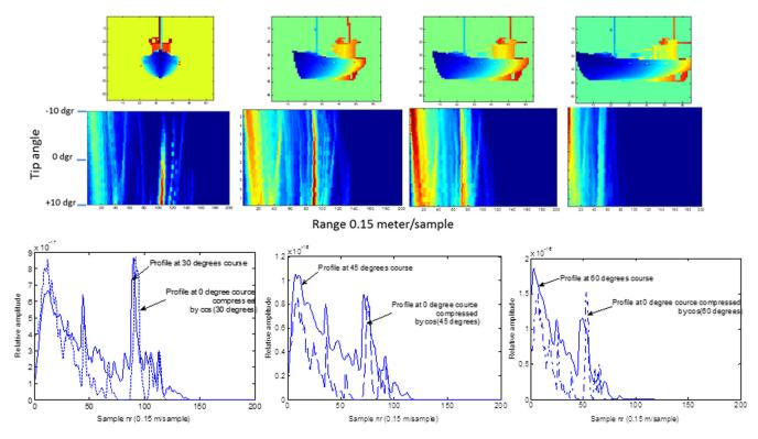
**Fig. 6** The top row shows the range profiles for the fishing boat observed at different courses and tip angles. The bottom row is a comparison of different profiles at courses  $\theta = 30$ , 45, and 60 deg with the  $\cos(\theta)$  compensated range profile at  $\theta = 0$ .
