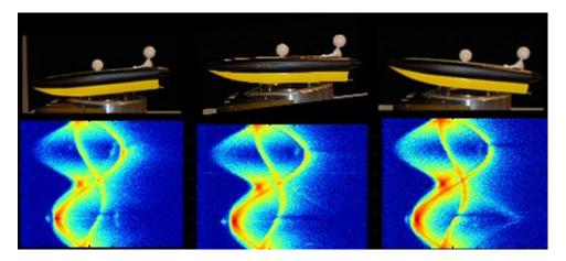
Fig. 11 Tipping the row boat  $\pm 6$  deg and the associated range profiles for 341 angles.
