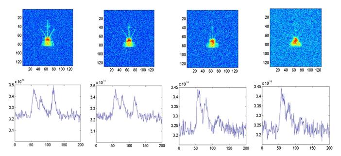
**Fig. 23** Examples of waveforms for increasing turbulence for boat no. 2 at 8-km range. Note the increasing blur in the intensity images and relative change in the peak amplitudes. The peak positions are relatively constant. The turbulence levels were from left to right  $C_n^2 = 10^{-15}$ ,  $10^{-14}$ ,  $10^{-13}$ , and  $5 \times 10^{-13}$  m<sup>-2/3</sup>, respectively.
