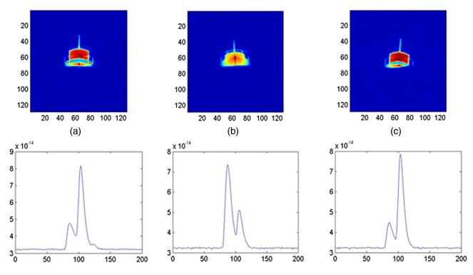
Fig. 21 Examples of different waveforms and boat aspects during a sea state corresponding to a wind velocity of 10 m/s. The time difference between the sampled waveforms is 1 s. Boat no. 2 at a range of 3 km.
