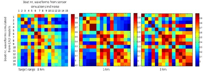
Fig. 16 The correlation matrix between boat profiles with no detector noise and those from the simulated sensor including noise. The separation capability is increasing with increasing signal-to-noise ratio (shorter ranges).
