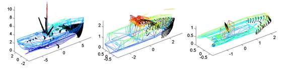
Fig. 25 CAD matching with correct model for (a) boat 2, (b) 9, and (c) 14, target range 3 km. Number of target samples: 3402, 803, and 199, respectively.
