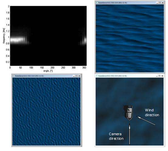
**Fig. 1** One of the wave situations simulated in the paper, where the wind speed is set to 10 m/s. (a) The spectrum, where the angle axis is defined as 0 deg when wind blows from east/right. White values correspond to high wave amplitudes. (b) Enlargement of the waves, while (c) is the same waves seen from the top. (d) The definition of the wind direction compared to the camera direction.
