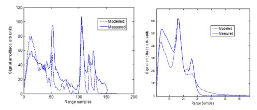
Fig. 12 Comparison between measured and modeled range profiles of the fishing boat. (a) Boat with course 0 deg, 0 tip angle. (b) Side view at 90 deg.
