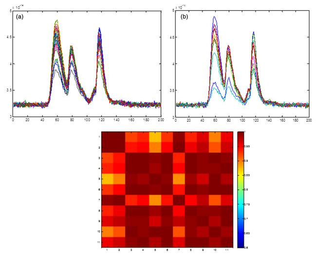
**Fig. 20** A series of waveforms for different beam jitter. (a) The rms jitter is assumed to be =1/10 of the FOV or 0.256 mrad. (b) The corresponding with a beam jitter = 1/3 FOV = 0.85 mrad. Above the shape of waveforms and below the corresponding correlation matrix between the different waveforms. Note the color bar span from 0.8 to 1 for the correlation coefficient.
