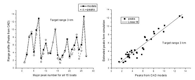
**Fig. 17** (a) A comparison between the peaks "extracted by hand" from the CAD models and those obtained from the simulated waveforms. Target range 3 km and low turbulence ( $C_n^2 = 10^{-15} \text{ m}^{-2/3}$ ). The peaks originate from the major peaks from all the 15 boats at a range of 3 km. (b) A regression line between the simulated data and that derived from the CAD model directly. The correlation coefficient was 0.96.
