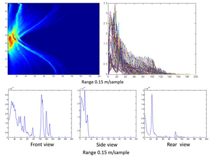
Fig. 4 The same as Fig. 3 but with an increased resolution by a factor of 5 (pulse length 3 ns and 24-m boat length). The signature will in this case contain many more details as expected.
