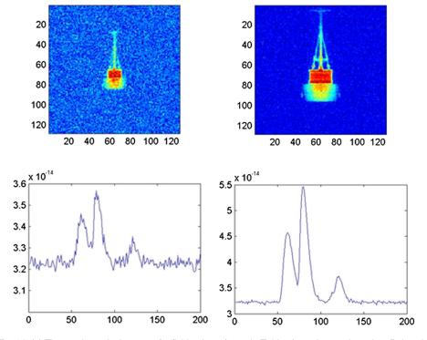
**Fig. 14** (a) The two intensity images of a fishing boat (no. 5 in Table 1) as observed at 8 km. Below the corresponding range waveform sampled at 1 ns/unit of the return energy (in joules). (b) The corresponding at 5-km range.
