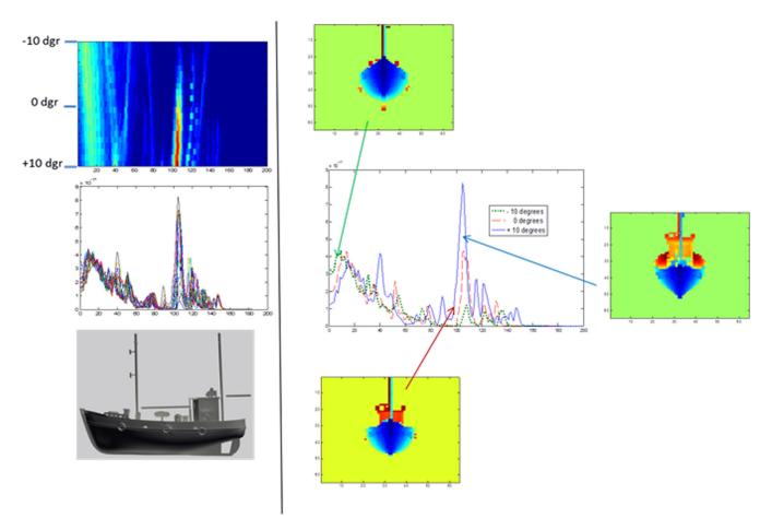
Fig. 5 Illustration of the change in range profile in the front perspective when the boat is tipped  $\pm 10$  deg. The change can be rather large as some of the structure will have a different visibility for the different slopes.
