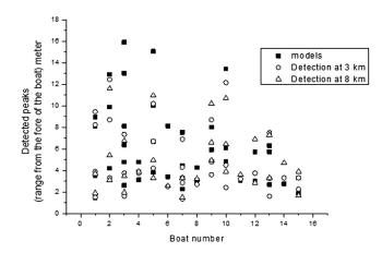
Fig. 18 Detected peaks for each boat derived directly from the CAD models as well as from simulated waveforms for the boats at 3 and 8 km range.
