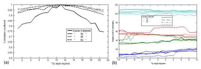
**Fig. 7** (a) Correlation for the range profiles at different tip angles and for different courses. The correlations are high especially at oblique courses. (b) The positions of the 4 highest peaks in the profile for different tip angles and courses [including the  $\cos(\theta)$  correction factor].
