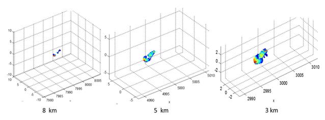
Fig. 24 Example of detected 3-D point clouds for boat no. 9 approaching toward the sensor at different ranges.
