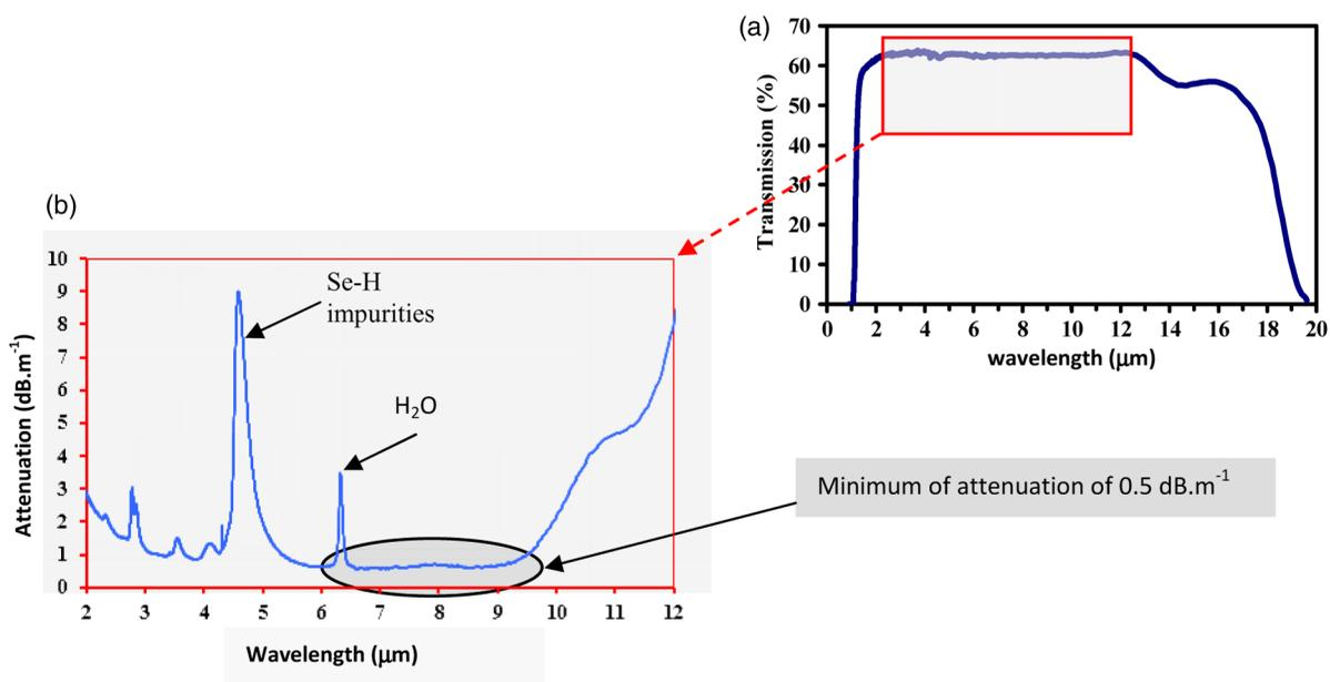
**Fig. 1** (a) Transmission window for a bulk of  $\text{Te}_2\text{As}_3\text{Se}_5$  glass (thickness 1 mm) together with the attenuation curve of the TAS glass fiber (b).<sup>40</sup>
