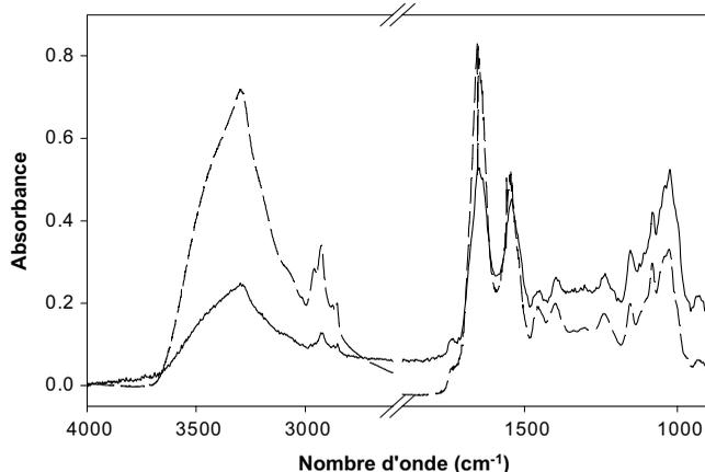
**Fig. 3** Comparison between the mouse liver spectra recorded in transmission mode (solid line) and with the optical fiber (dashed line).<sup>42</sup>
