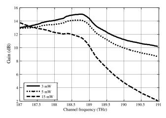
Fig. 3 Gain spectra (with  $P_{\rm in}$  = 3,5, and 15 mW) of Raman-EDFA HOA.  $^{42}$
