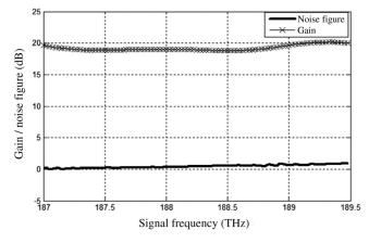
Fig. 4 Gain and noise figure characterization of optimized EDF-Raman HOA.  $^{\rm 44}$
