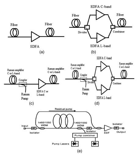
**Fig. 2** Architectures of inline optical and hybrid optical amplifiers: (a) a EDFA; (b) dual C-or L-band EDFAs in parallel configuration; (c) C + L band Raman-EDFA Hybrid optical amplifiers (HOA) in cascaded configuration; and (d) Raman-EDFA HOA, where the EDFAs are used in parallel configuration (CMB: combiner, DIV: divider); (e) cost effective Raman-EDFA HOA with residual pump.<sup>9</sup>
