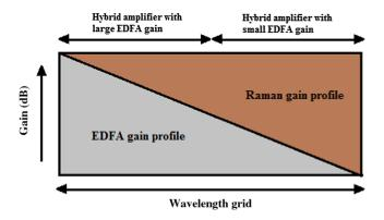
Fig. 1 General presentation of gain partitioning in hybrid Ramanerbium doped fiber amplifier (EDFA).
