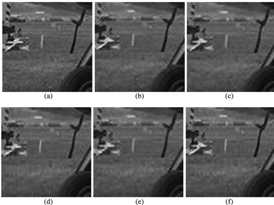
**Fig. 7** Cropped regions after deinterlacing: (a) original, (b) edge-based line average (ELA), (c) gradient-guided deinterlacing (GGD), (d) LCIM, (e) moving least-squares method (MLSM), and (f) the proposed method.
