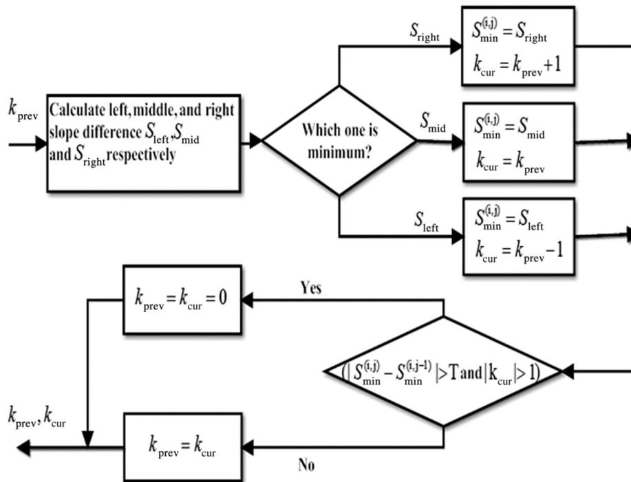
Fig. 1 Flow chart of the edge slope tracing (EST) process.
