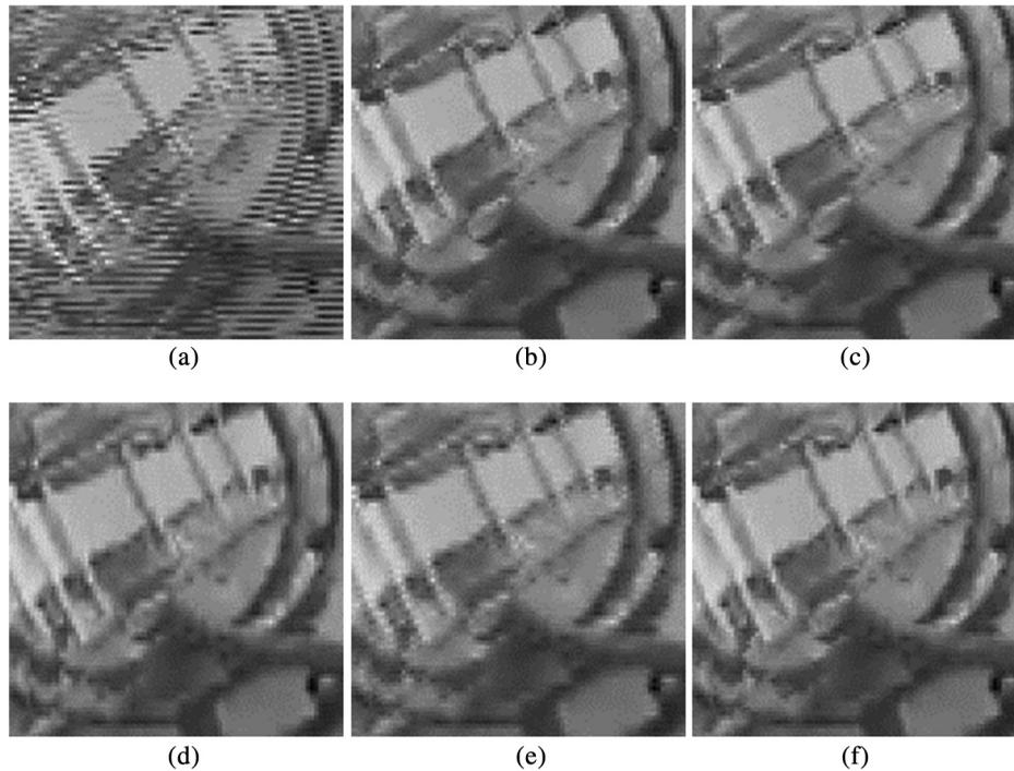
**Fig. 12** Cropped regions after deinterlacing: (a) original interlaced frame, (b) ELA, (c) GGD, (d) LCIM, (e) MLSM, and (f) the proposed method.
