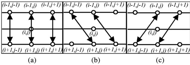
**Fig. 5** Differences for determining  $\pm 75$  or  $90$  deg slope: (a)  $d_1$ , (b)  $d_2$ , and (c)  $d_3$ .
