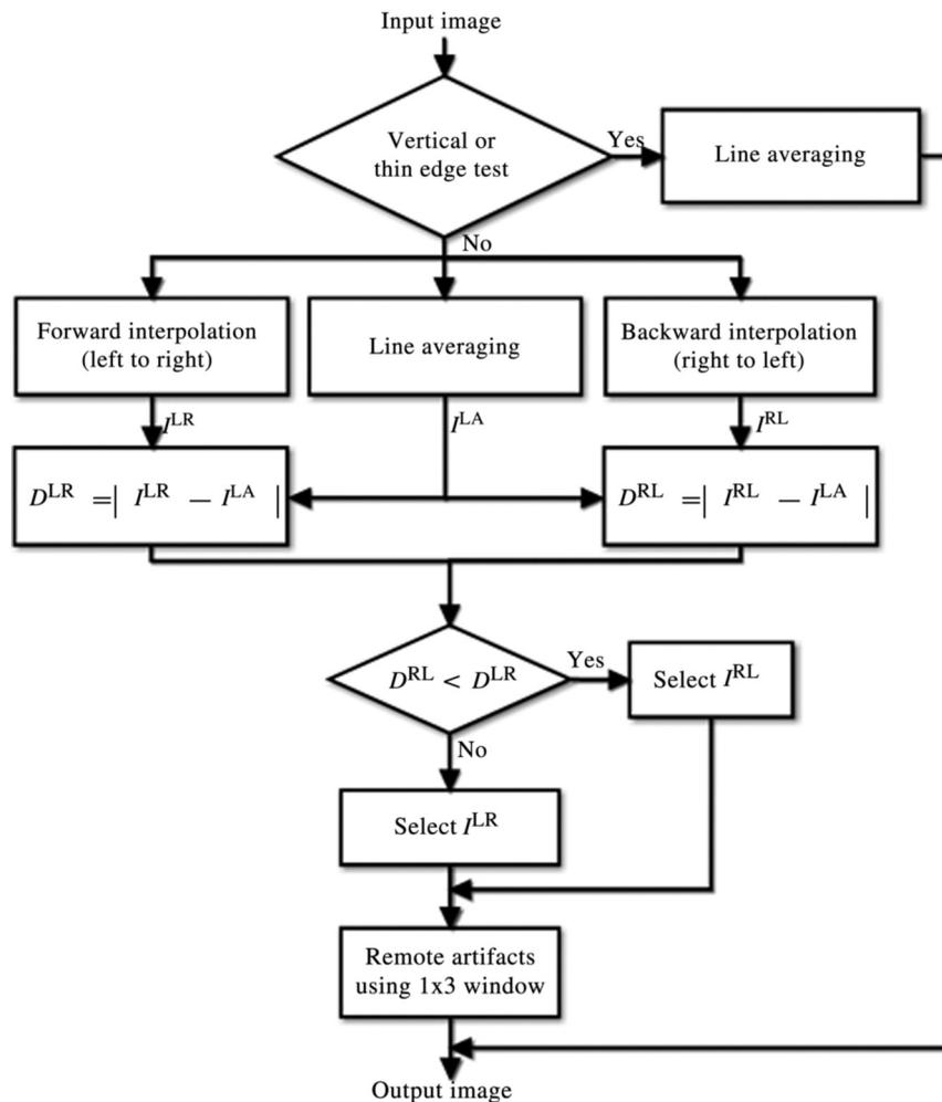
Fig. 4 Flow chart of the proposed interpolation method.
