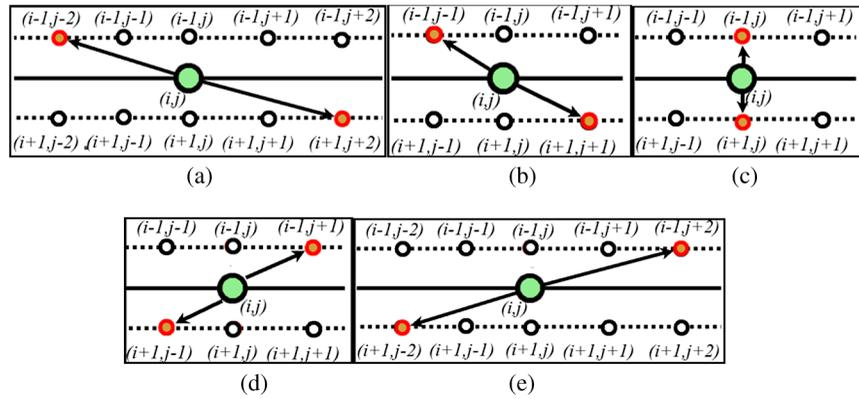
Fig. 3 Examples of slope-based interpolation using different slopes: (a) -2, (b) -1, (c) 0, (d) 1, and (e) 2.
