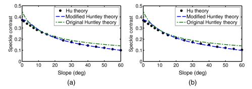
**Fig. 3** Comparison of Hu, Huntley, and modified Huntley equations when both slope and roughness reduce speckle. In (a), a Gaussian spectrum is used, while a Lorentzian is used in (b). The modified Huntley matches Hu's theory very well with a region of slightly higher error for slopes between 2 deg and 10 deg. Conditions: 0.3 m aperture, 5 km range, 1  $\mu$ m wavelength, 1 mm coherence length, and 1 mm surface height standard deviation.
