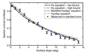
Fig. 5 Comparison of measured speckle contrast with both Hu and Huntley theory. The error bounds about the measurements are standard error of the mean, sometimes called 68% confidence intervals. Note that 11 of 16 of those error bounds encompass Hu's theory, about the expected ratio assuming Hu's theory is valid.
