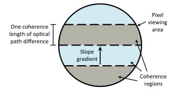
**Fig. 1** A geometrically approximated circular pixel viewing area on target showing four shaded coherence zones. The zones form due to the slope of the surface and have long dimensions perpendicular to the slope gradient. Each coherence zone is separated by one coherence length of optical path difference.
