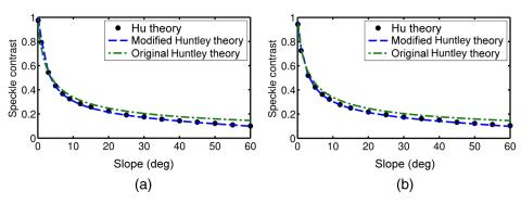
**Fig. 2** Comparison of Hu, Huntley, and modified Huntley equations. (a) A Gaussian spectrum and (b) a Lorentzian. The Hu and modified Huntley equations agree well, while the original Huntley shows considerable disagreement at large slope angles. Conditions: 0.3 m aperture, 5 km range, 1  $\mu$ m wavelength, 1 mm coherence length, and 5  $\mu$ m surface height standard deviation.
